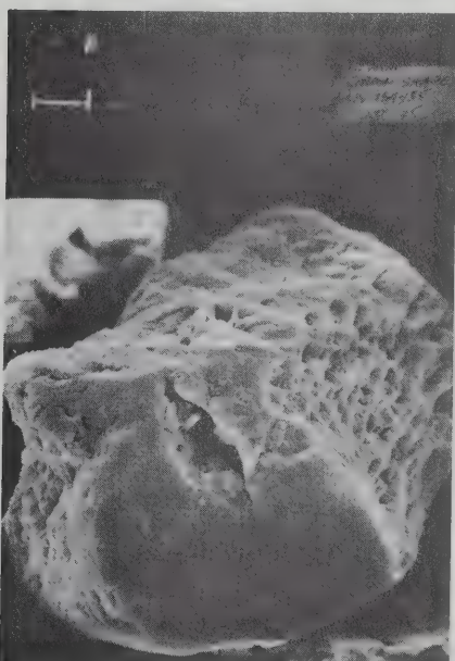
7.6c McMurray Formation Deep pit. The concavities on the top and the right are contact points typical of interpenetrative sands.
